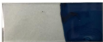
Fig. 1 Hydrogen bronze film after 100 s of electrodeposition on a 1" x 3" ITO slide https://doi.org/10.30799/jtfr.025.20040101
